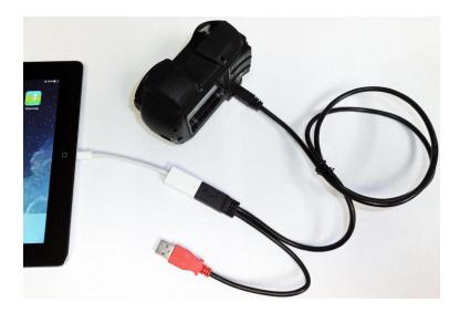
USB Y Cable with two USB-A on one end (power + data) and Micro-B on the other end. The above cable is made by StarTech, but other brands are available.
